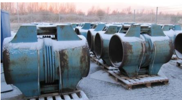
The compensators prior to repair
